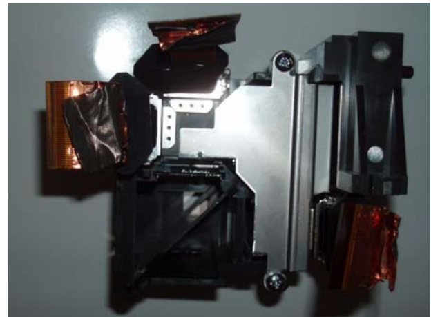
Fig. 3 Color recombination unit with LCOS panels.
