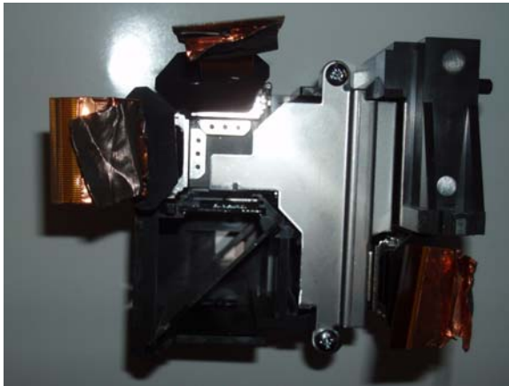
Figure 4. A commercial color recombination unit with LCOS panels.
