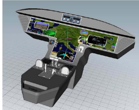
Figure 7. Artist impression of the single panel display integrated in the cockpit.
