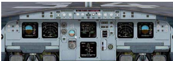
Figure 1. Modern cockpit of an Airbus A320 aircraft, featuring 6 larger size LCD displays.
